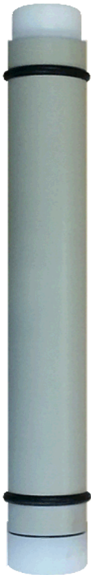
Acoustic logger (600 x 95mm)
